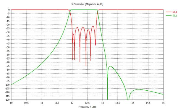
Figure 5: Coaxial filter and frequency response computed by CST
