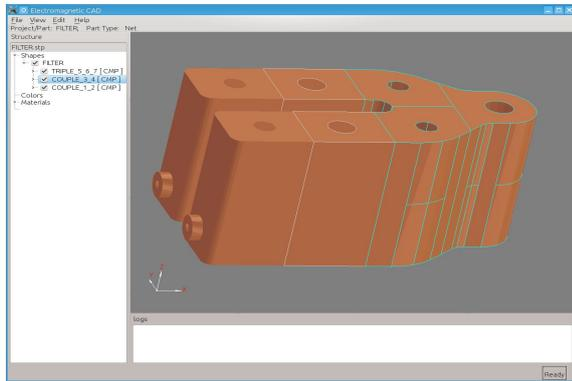
Figure 2: Coaxial filter imported in EmCAD
