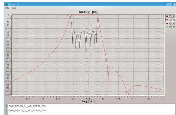
Figure 4: Frequency response computed by EmCAD
