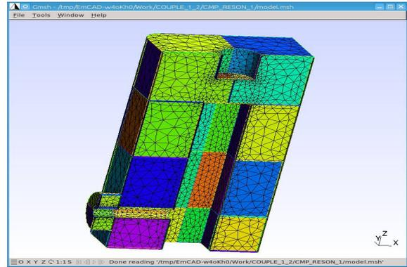
Figure 3: Domain decomposition and meshing of first resonator
