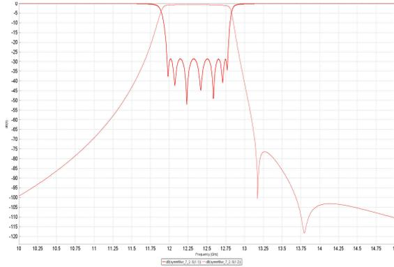
Figure 1: Seventh order ideal resonator circuit and related frequency response
